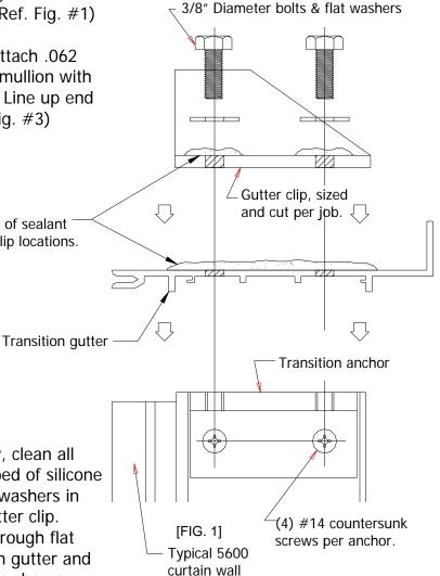
C.) Prior to setting clip assembly, clean all metal surfaces and lay in a bed of silicone sealant at clip location. Set washers in silicone sealant on top of gutter clip. Insert 3/8" diameter bolts through flat washer, gutter clip, transition gutter and secure to transition anchor as shown. (Ref. Fig. #1 & #2)
