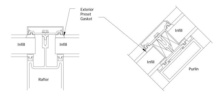
E.) Refer to Fig. #14 to insure that sealant is at rafter to purlin joinery as illustrated.
