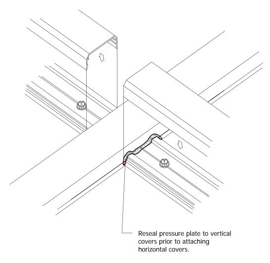
D.) Center horizontal snap cover in opening; engage one side, then use block and mallet to engage opposite side. Gaps at ends should be equalized, and are provided to allow installation, to allow thermal movement, and provide weepage.
