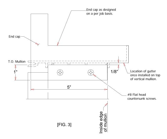
A.) Seal joint between gutter and end cap as shown. When jamb condition is exposed (end wall condition), use a 3/8" diameter X 3" long countersunk bolt to secure the lower rafter clip to the gutter clip. This will allow for overlap of flashing as designed.
