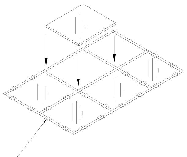
Note: Temporary Glazing Retainers are available from EFCO. These retainers are considered an extra, and can be provided at customer's request.
