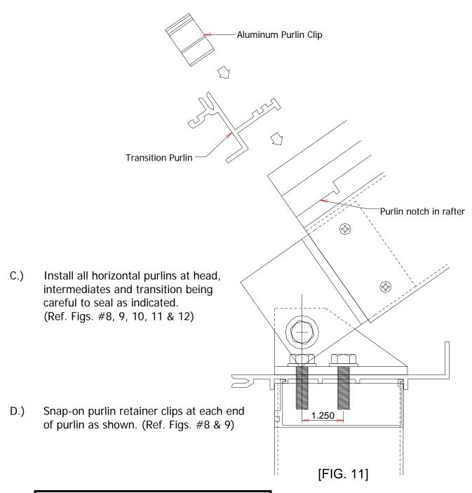
Note: Make sure the clips are secured in position in order to hold down purlins.
